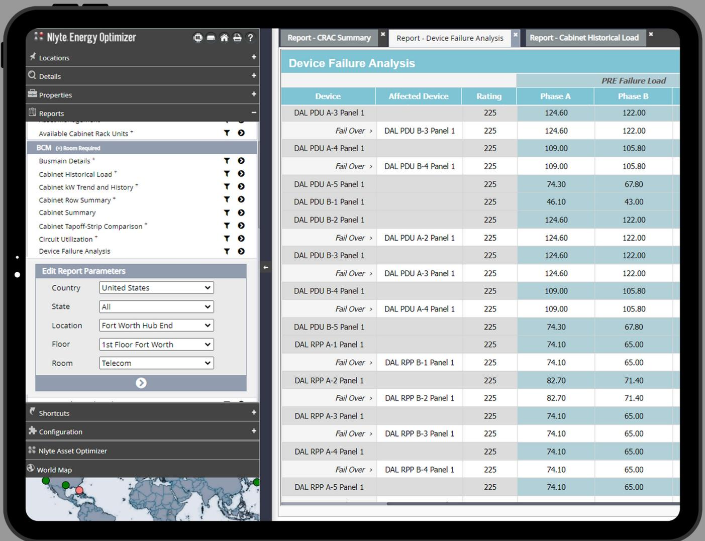
The Nlyte Device Failure Analysis report in the Nlyte Energy Optimizer (NEO) solution focuses on predicting and preventing potential equipment failures in data centers. The report utilizes advanced algorithms and historical data to analyze the performance and health of devices within the data center, identifying trends and patterns that may indicate a higher likelihood of failure.
