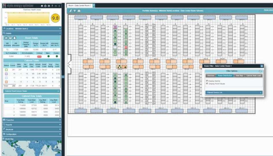
Floor plan within Nlyte Energy Optimizer and the highlighted rack V-PDU usage
