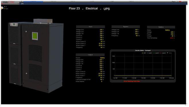
Figure 3: IDCM provides insight into the existing battery life on a UPS and can provide sufficient warning time in advance of failure for workloads to be properly and safely migrated.
