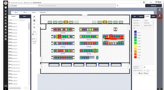
Figure 4: The joint Nlyte and Automated Logic IDCM solution allows users to visualize where they have remaining cooling capacity based on commitments that have already been made against thresholds.
