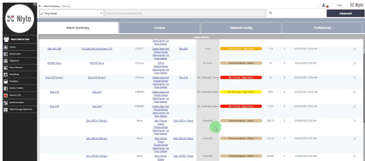
Figure 18: Example Alarm summary with criticality indicated by color.
