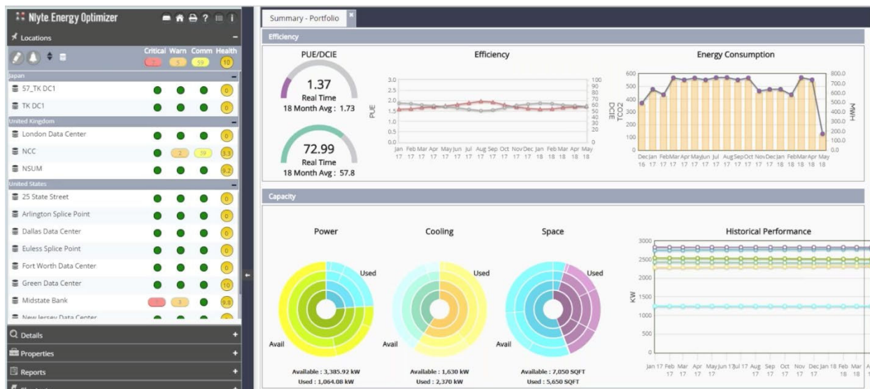
Figure 9: Example Power Management, PUE
